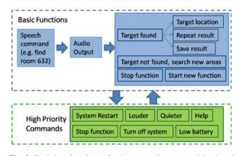
**Fig. 9** Basic interface design for the proposed computer vision-based indoor wayfinding system by using speech commands. The high priority commands can be used at any time to overwrite the basic functions
